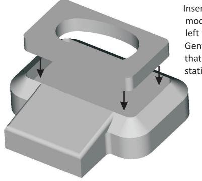
Insert the inlay such that the mod's buttons will show to the left when plugged in. Gently press the inlay such that it fits flush in the charger station.
