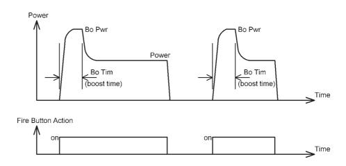
The dynamic boost operation is illustrated on the top of the next page: Whenever the fire button and the plus button are pressed at the same time, the boost power is selected and applied to the coil. Otherwise just the selected power is applied.
