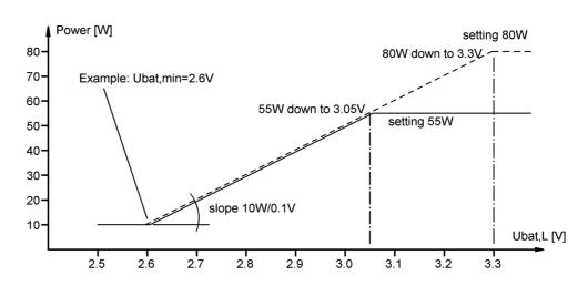
At UBatMin+ 0.7V a power reduction is activated depending on the actual power setting. The reduction starts when the power selected hits the slope from Ubat,min@10W to Ubat,min+0.7V@80W as shown in the diagram above.
