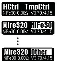
In this mode the mod will regulate the temperature of the coil to the pre-set value, except the power setting is too low to achieve the temperature. So please note to adjust the power setting to a value high enough, if you choose temperature controlled vaping. Otherwise the temperature regulation changes to a temperature limitation mode.
