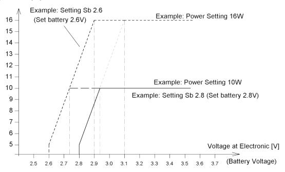
In the diagram, two example settings of the parameter Sb are shown. With a setting of Sb to 2.6V, for example, and a chosen power of 16W, the power reduction starts at a battery voltage (under load) of about 2.9V; this is the dashed line in the diagram. For the second example, Sb is set to 2.8V and the power is 10W. In this case the reduction starts at about 2.93V (bold line in the diagram). With Sb=2.6V and 10W, the power limitation would start at a voltage of about 2.73V (long dashed line).
